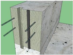
Insure the waterbar is properly placed in the centre of wall or kicker according to instruction and secured into position and has at least 75 mm of cover.
